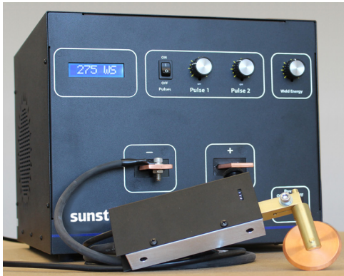
Figure 8.1. Roll Spot hand held attachment example. This configuration requires an upgrade.
