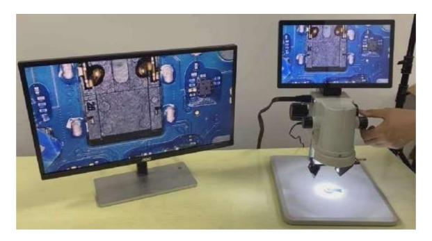
The  $ProZoom\ Digi\ 9M-3D$  integrated zoom optical module with high definition camera. It can be conveniently used in a narrow and small space. According to ergonomic principles, its internal optical corner design and angle adjustment of the display screen, allow the operator to look at the display in a flat view. Through the HDMI HD interface, it can connect to another display simultaneously. USB interface to connect to PC.
