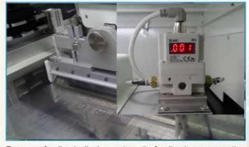
Pressure feedback display, automatic feedback compensation, pressure equalization, printing process stability extended stencil, scraper life
