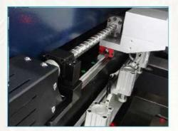
The squeegees transportation adopts the ball-screw with the servo direct connection, This robust design ensures the highest degree of reliability & repeatability.
