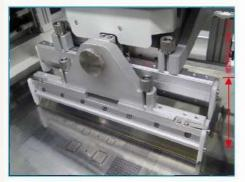
The Patent self-developed "electrical&air Pressure combined type" printing head ensures the printing precision after printing and as well as the solder paste molding and solder paste volume.
