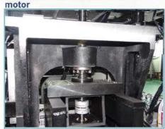
The lifing table is directly connected with servo motor and ball screw to precisely control the precision of lifting position and snap-off precision. improve the movement rigidity. BTB
