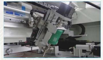
The system automatically monitors the roller height of solder paste on the stencil in real time, and intelligently replenishes solder paste automatically. The amount of solder paste discharge is controlled by air pressure and diameter of solder paste outlet. Motor translation plus solder paste and the length is programmable.
