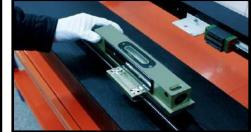
X&Y Guide Rail Testing
