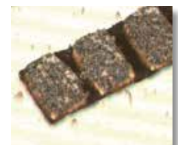
2D+3D Image with clear low bridge defect
