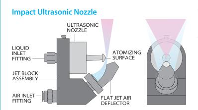
The EZ-Flux system can either be installed internally in your wave solder machine or is available as a stand-alone unit.
