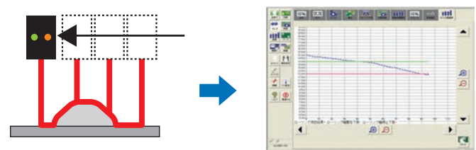
Measures rolling width of solder
